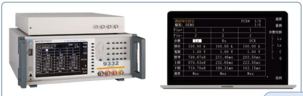
Using LCR Meter to check Inductor Impedance characteristics of FPC Coil.
