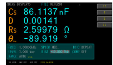
Applying a 40V DC Bias voltage, the capacitance value decreases to 86.1nF
