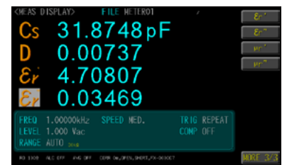
Monitoring \epsilon_r' / \epsilon_r'' in Meter Mode
